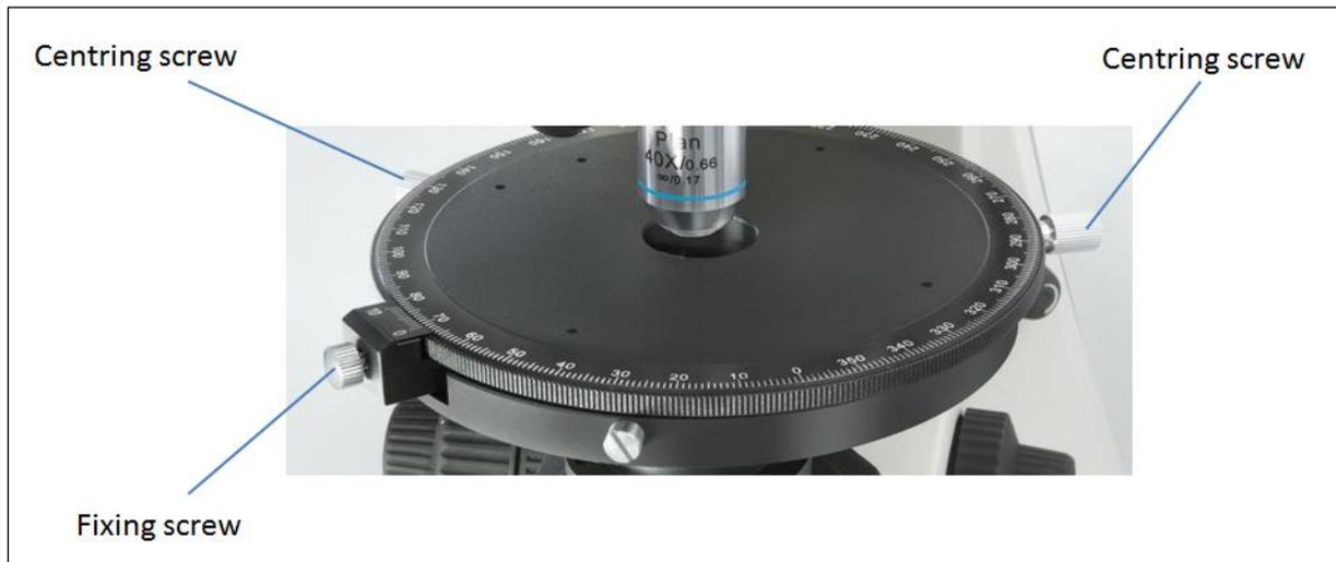
1. Bring the 10x objective into beam path.
