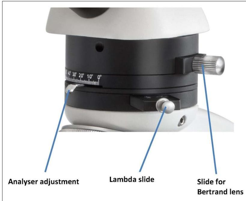
The setting of the analyser now has to be done with help of the according lever, which needs to display 0°. As a result the orthogonality between polariser and analyser, which is required for common polarisation applications, is ensured. An indication for this orthogonality is the maximum obscuration, which can be thereby observed in the field of view.
